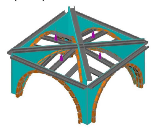
fix the hangers to the centre of the upper arches 80cm from the perimetral walls, depending on the room's dimensions
