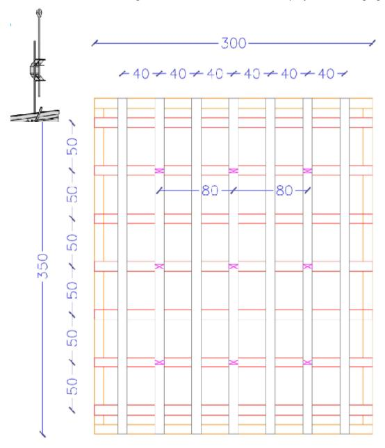
proceed with the plasterboard laying (thickness 6mm/10mm), which will find a continuous surface for optimum shaping
