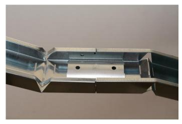
connect the CONCAV&CONVEX / CONCAVEX Curving Studs to the primary metal framework with channel hangers, with an interaxle spacing of 30cm (or 40cm, depending on the radius of the curvature)
